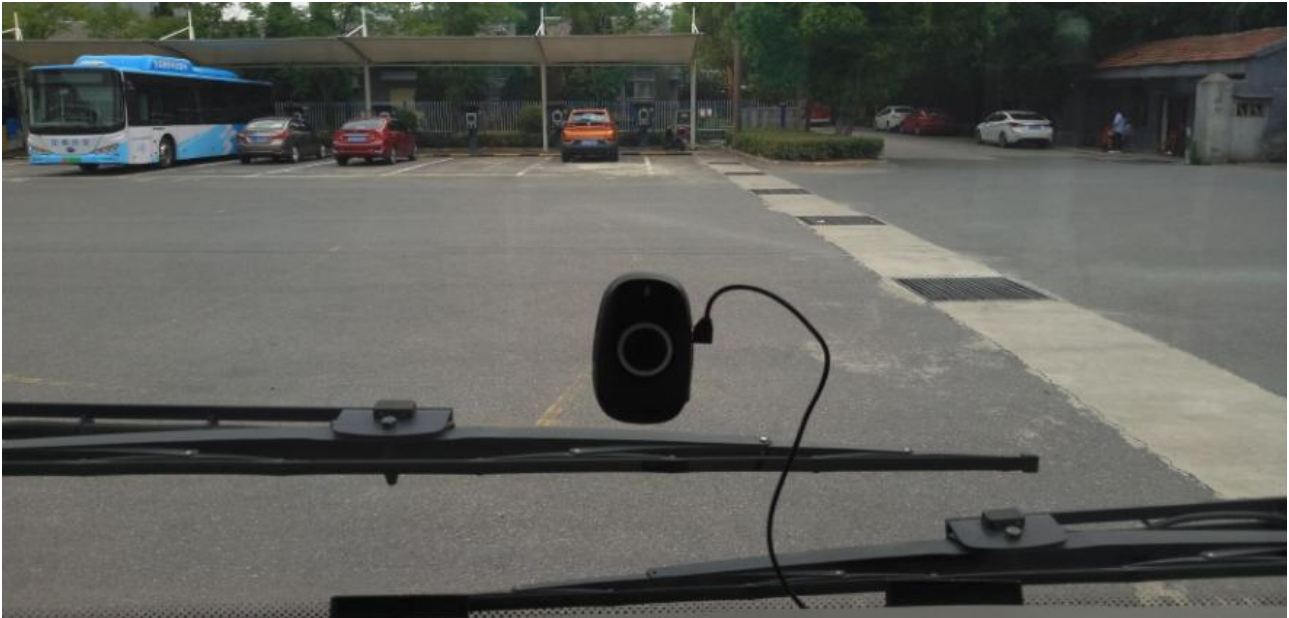
Camera installation of larger vehicles
